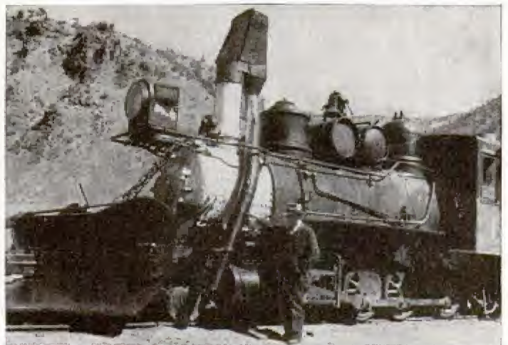
The old-type narrow gauge engine, below, has cinder collector
